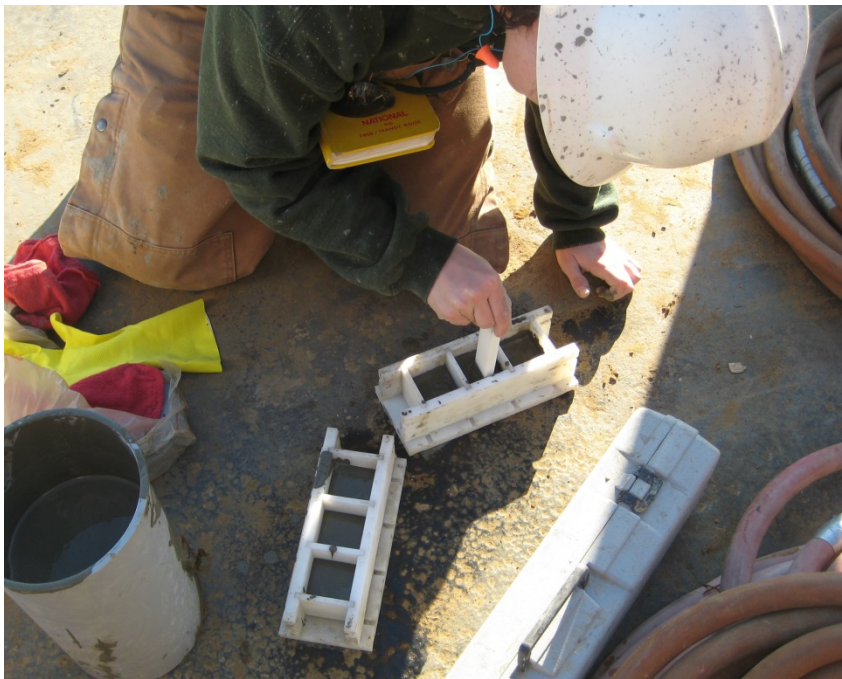
Figure 3.6: Photo. Molding grout cubes for strength verification. Photograph courtesy of Schnabel Engineering.
